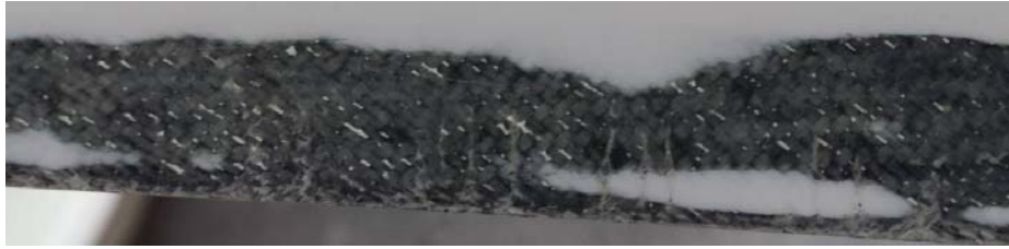
Figure 4. Crack damage in carbon fibre trailing edge.
