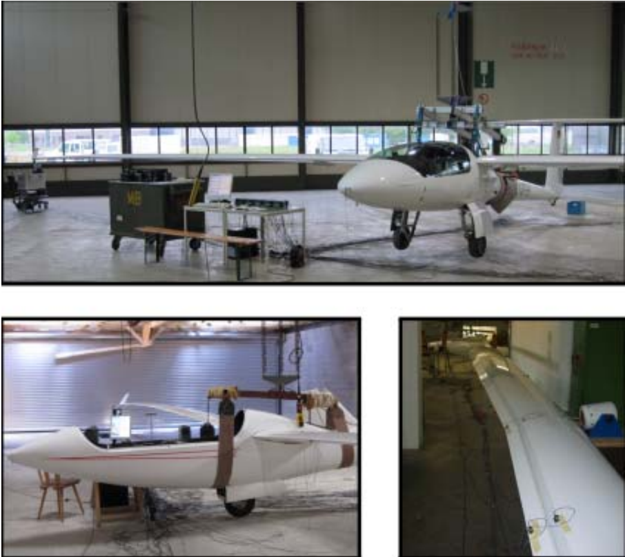
Figure 1. The test conditions during the ground vibration tests. (above Stemme S10-VT; bottom ASH25-EB28
