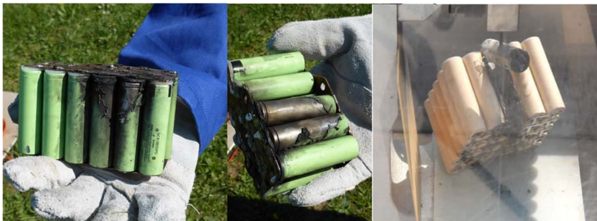
Fig.4 18650 cell packages after nail-tests
