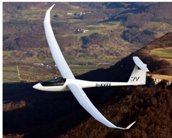
Fig. 1 The Schempp-Hirth “New” Ventus. MTOW, 600 kg; Wing Area, 10.32 m 2 ; Aspect Ratio, 29.9.
