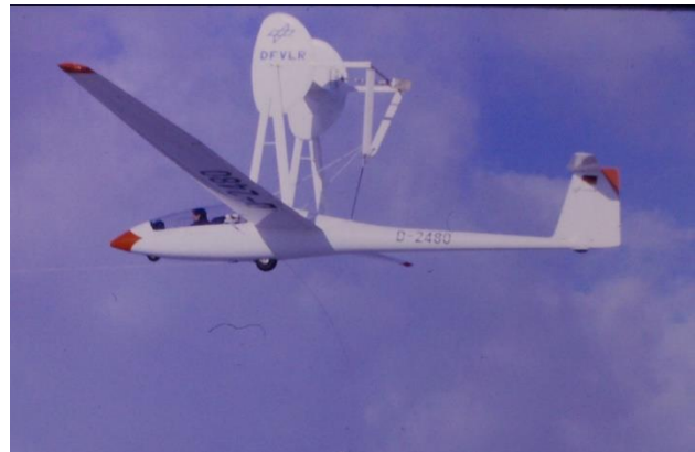
Figure 5: Janus with flying wind tunnel
