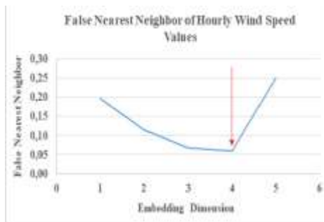
Figure 3.a. FNN of Hourly Wind Speed Data
